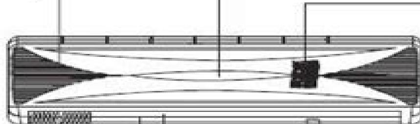
**Left/right air flow direction adjusting fin**
