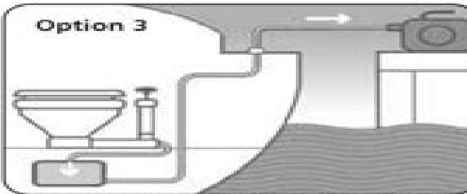
Collect waste in an on-board holding tank for discharge later to a Shore Station using a dockside suction pump or portable utility pump.
