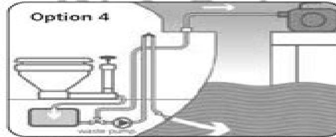
A combination of Option 2 and 3 to give you the flexibility of discharging waste whenever most convenient, and without the cost of a shore connection.
