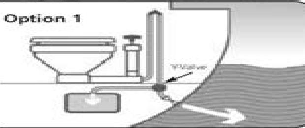
Discharge waste through a Y-valve directly into a non-polluted area or to a holding tank, when within the three mile limit, using the toilet's own pump and an anti-syphon loop.
