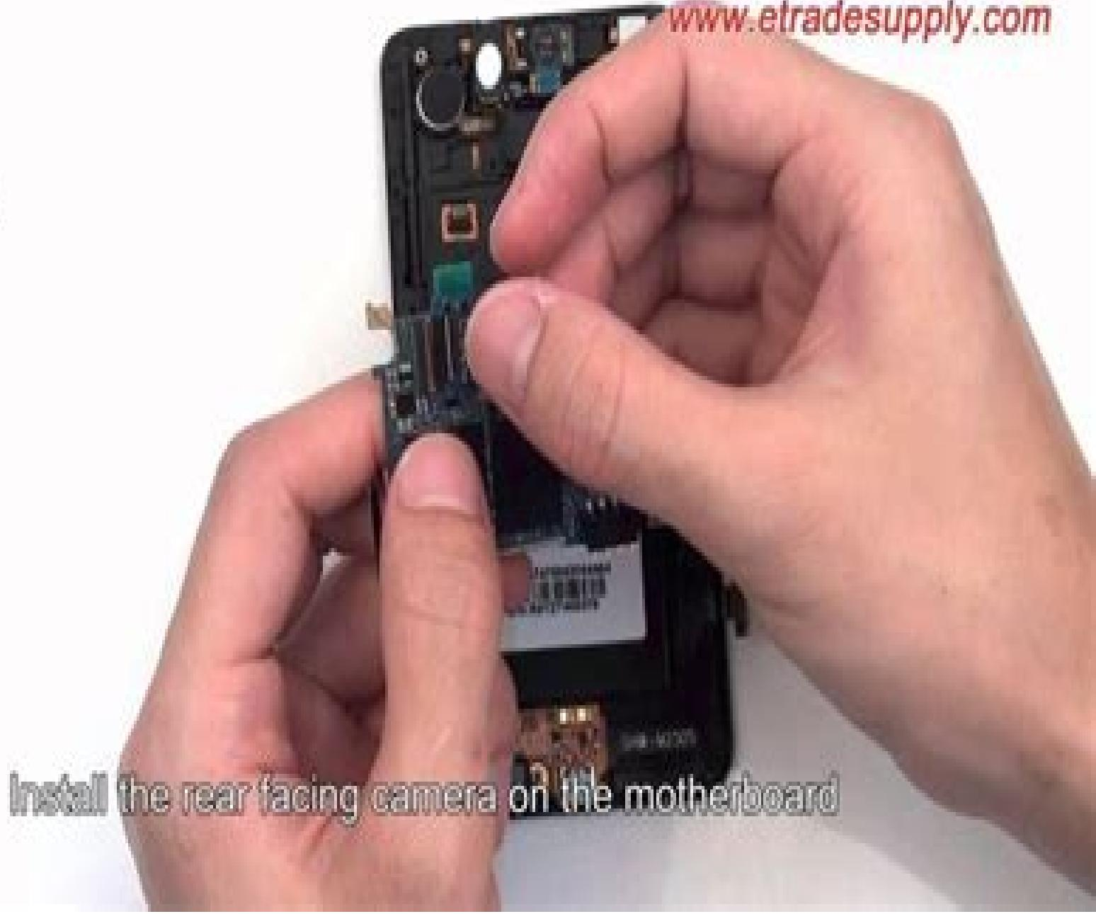
Install the rear facing camera on the motherboard
