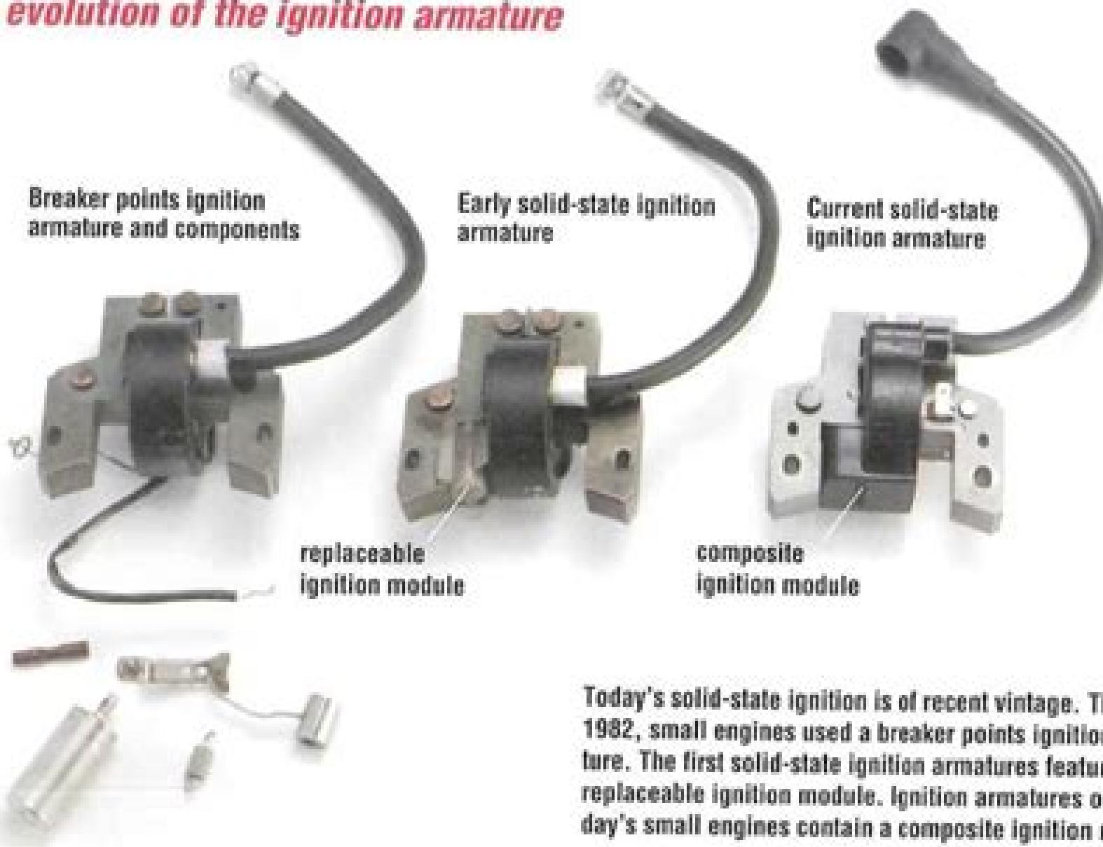
Today's solid-state ignition is of recent vintage. Through 1982, small engines used a breaker points ignition armature. The first solid-state ignition armatures featured a replaceable ignition module. Ignition armatures on today's small engines contain a composite ignition module.
