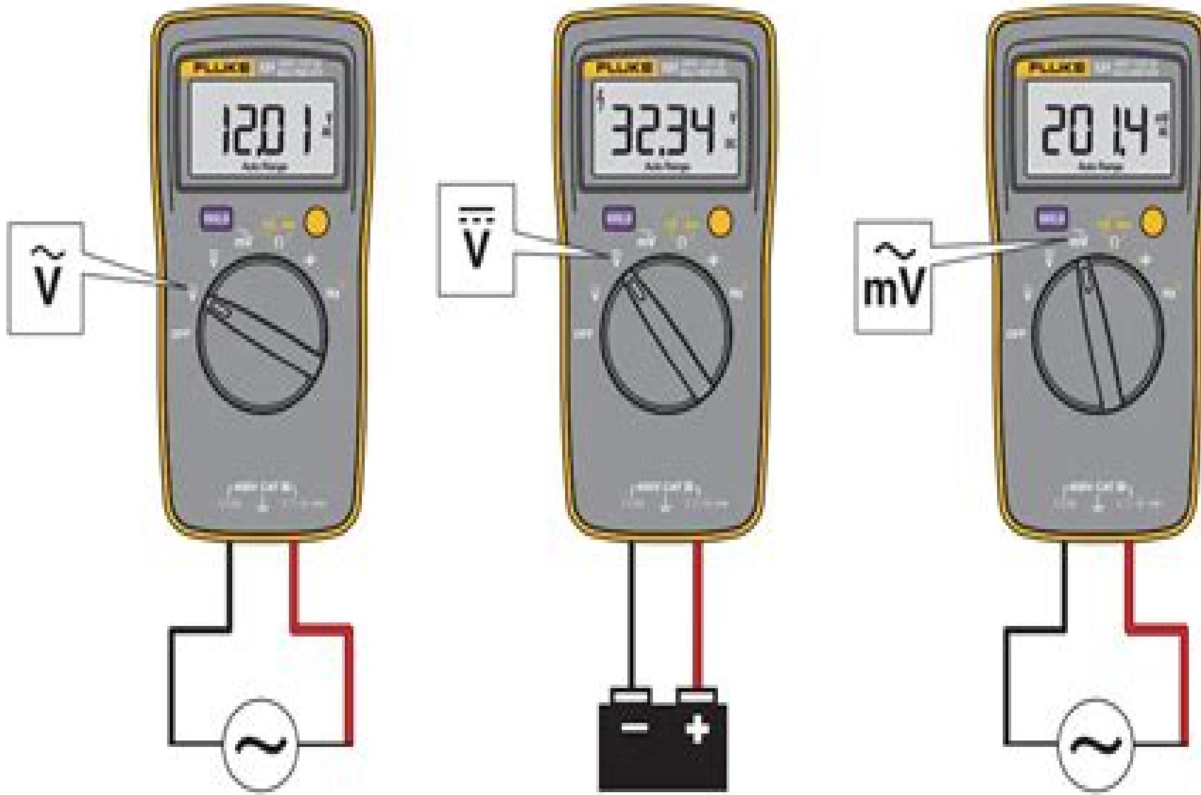
Figure 2. Measure AC and DC Voltage
