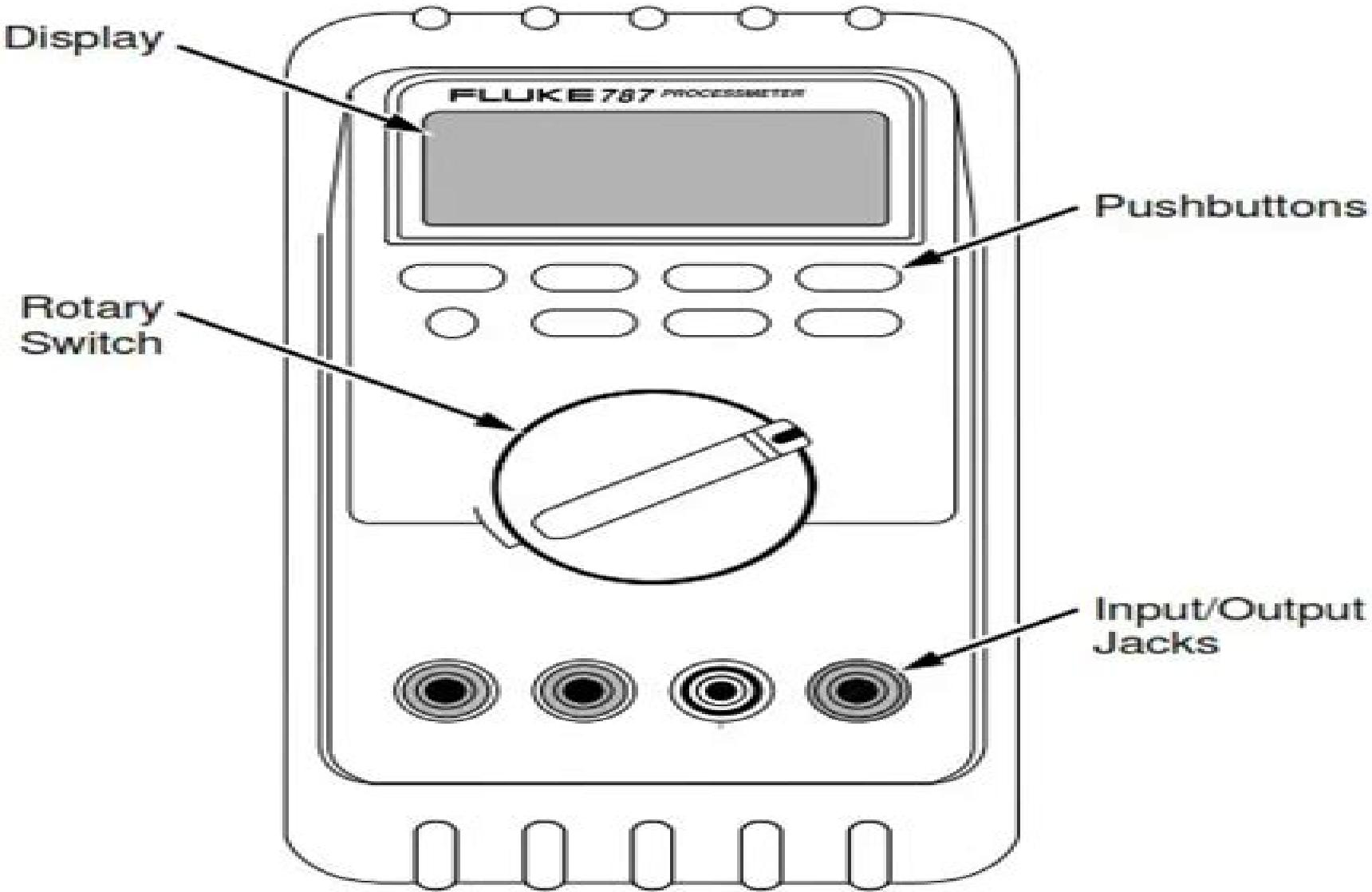
**Figure 1. Fluke 787 ProcessMeter**
