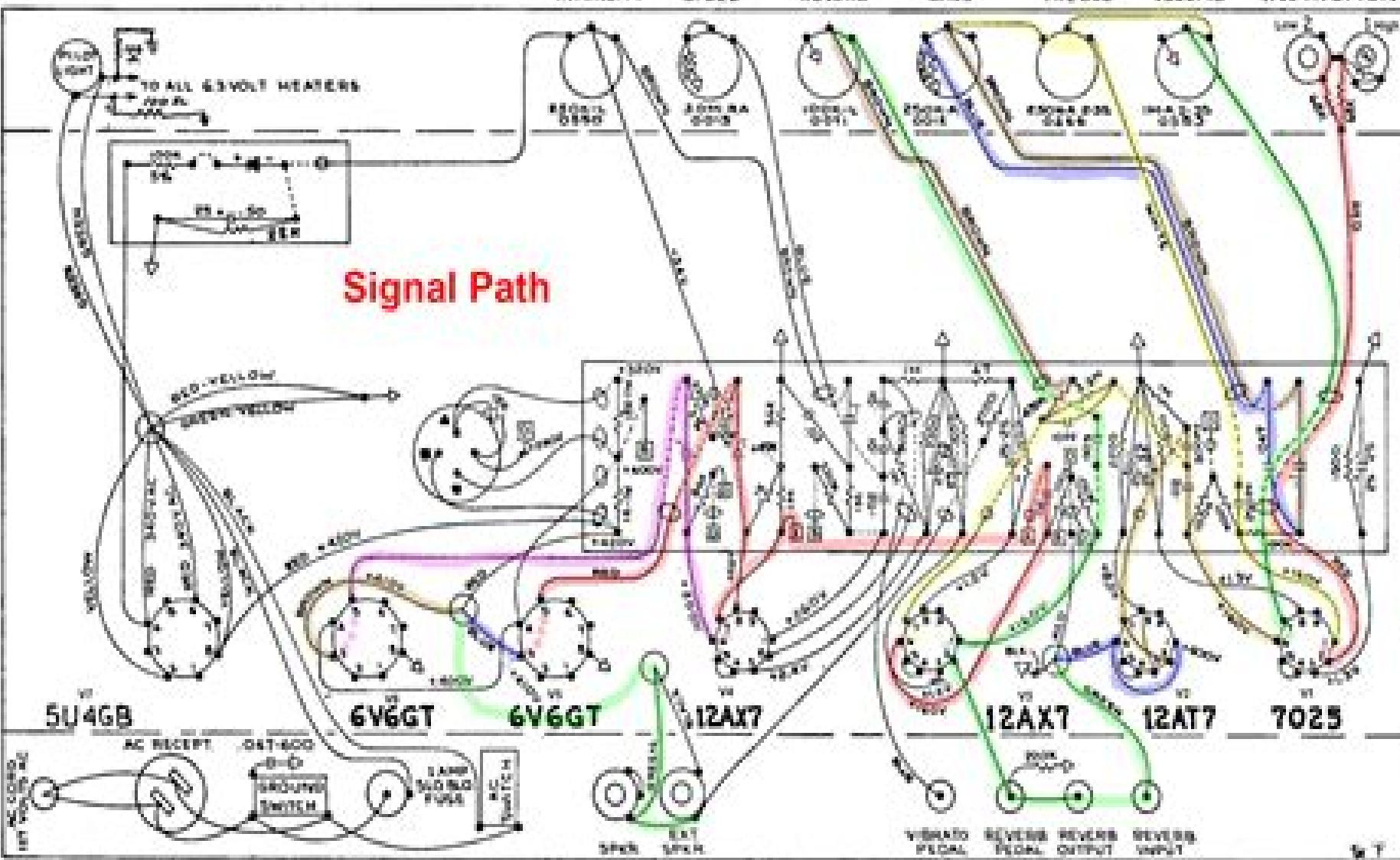
NOTE: ALL RESISTORS 1/2 WATT 5% TOLERANCE, IF NOT SPECIFIED
