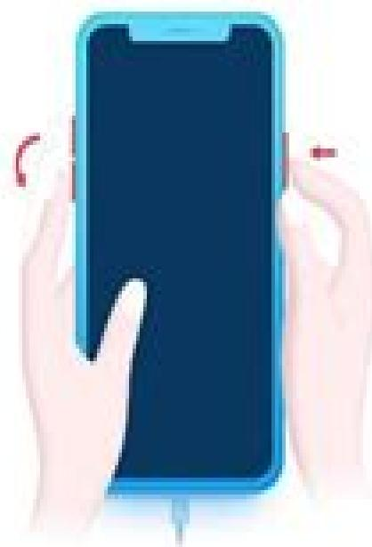
01 Connect your device to computer via USB cable. Quickly press the Volume Up button, then quickly press the Volume Down button. Next, press and hold the Power button even if the screen turns black.
