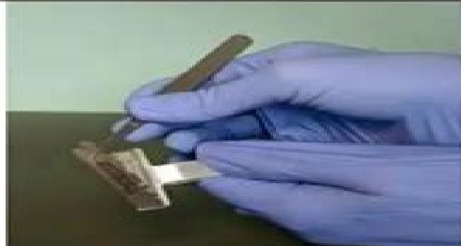
4 Soak the blade holder in the acetone bath for **5 minutes**. Wipe off any residual glue on the blade holder using a paper towel. It is critical to ensure all glue residue is removed before attaching a new blade.
