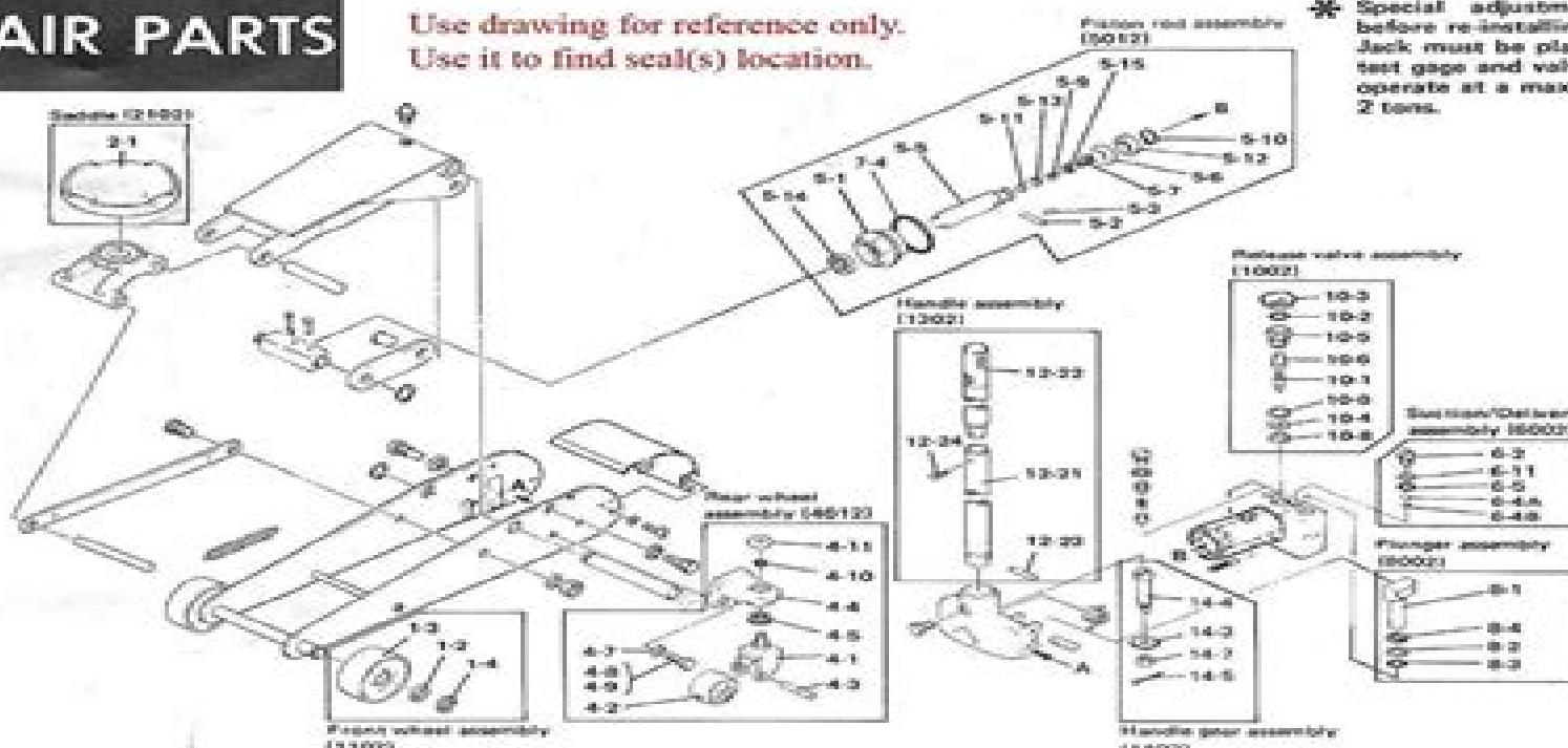
Special adjustment required before re-installing these parts. Jack must be placed on a load test gage and valve adjusted to operate at a maximum load of 2 tons.
