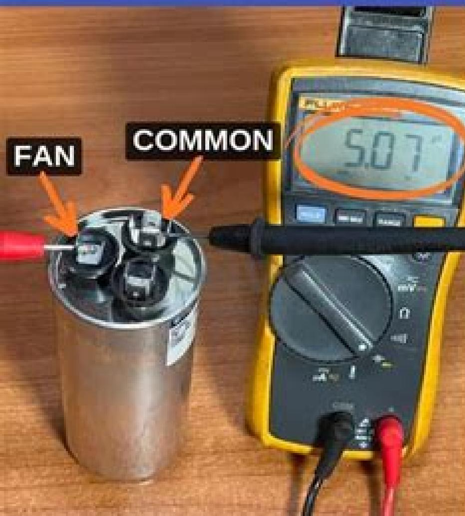
Hook up your multimeter leads to the **COMMON** and **FAN** terminals to measure the capacitance of the condenser fan's capacitor
