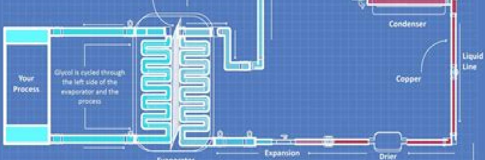
Metering Device/Expansion Valve drops the pressure of the refrigerant causing a drop in temperature. At this point, the refrigerant is a liquid/vapor mixture
