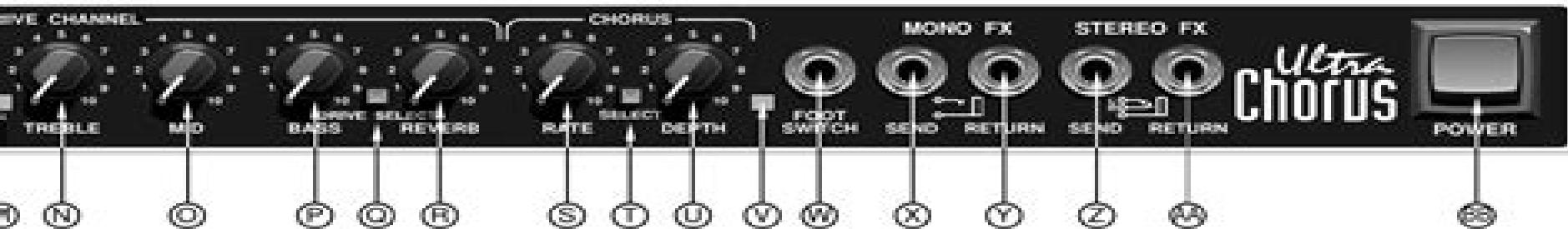
**U. DEPTH-** Adjusts the intensity of the chorus effect. A lower setting will introduce a subtle yet distinct effect, whereas a higher setting will create a more dramatic effect. With both the RATE (Item S) and DEPTH controls set midway or higher, a variety of vibrato/tremolo type effects can be achieved.
