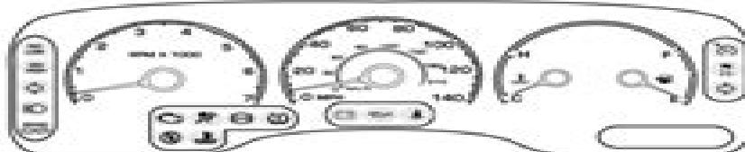
Warning lights and gauges can alert you to a vehicle condition that may become serious enough to cause expensive repairs. A warning light may illuminate when a problem exists with one of your vehicle's functions. Many lights will illuminate when you start your vehicle to make sure the bulb works. If any light remains on after starting the vehicle, have the respective system inspected immediately.
